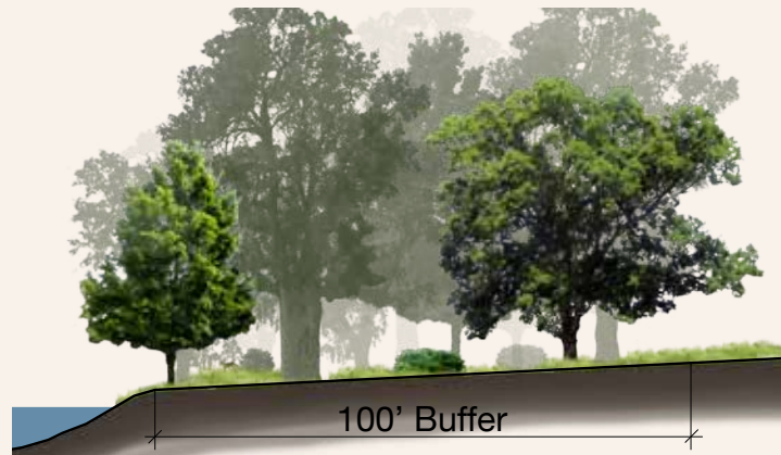
Figure 7 A forested riparian buffer is recommended to replace annual row crops at the top of streambanks.
