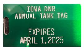
An annual tag listing "**April 1, 2025**" is required to receive fuel for tanks greater than 1100 gallons. The annual tag listing "April 1, 2025" must be on a UST fill ports to receive fuel deliveries.
