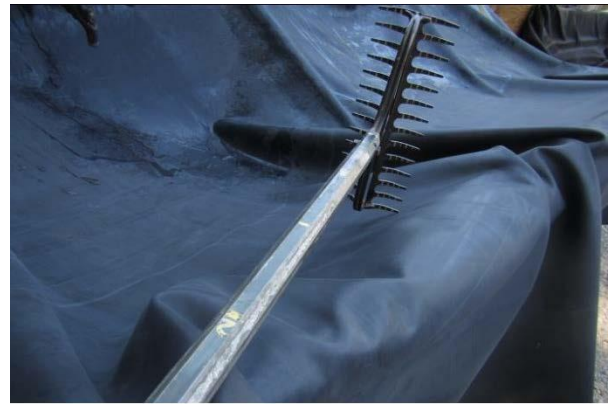
Figure 3. Floating hoop used to sample emergent, floating and floating leaved aquatic plants (left). Double-sided rake on an extendable pole used to sample submersed aquatic plants (right).
