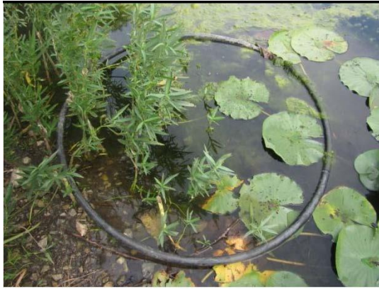
Figure 3. Floating hoop used to sample emergent, floating and floating leaved aquatic plants (left). Double-sided rake on an extendable pole used to sample submersed aquatic plants (right).
