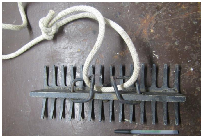
Figure 6. Weighted rake on a rope (WRR) for sampling at depths over 16 feet.
