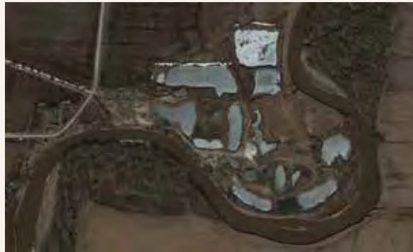
C4.B Obvious impact to the river channel, including an alternately over-wide and narrowed channel width, is visible 1.5 miles downstream of Oakland.
