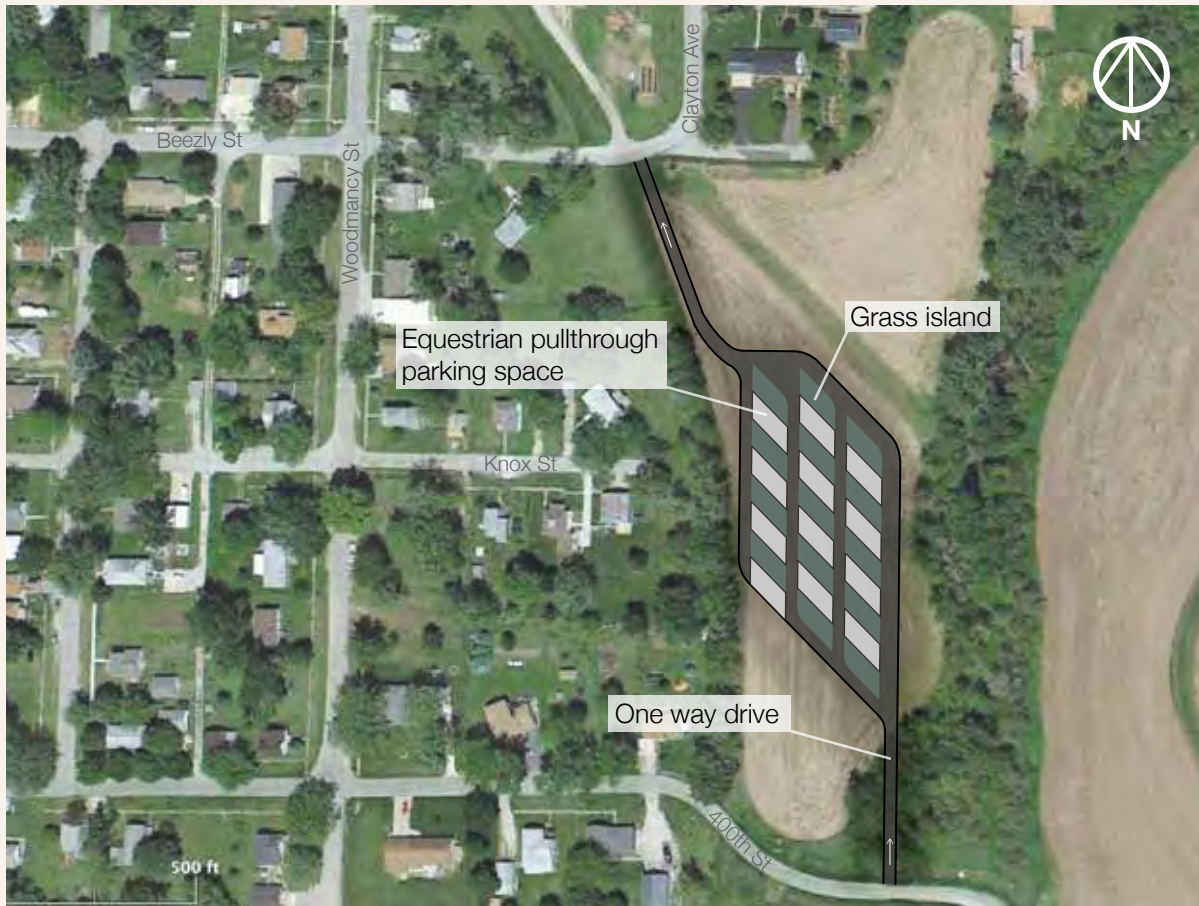
R4.C This equestrian parking area has pull-through parking for 12 truck + trailer units. Each parking area also has an adjacent grass area for set up.
